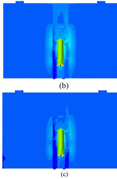
Fig. 3. Ex-core fluid and solid temperature distribution over axi-symmetric plane (XZ-plane). (a) 2 kg/s; (b) 4 kg/s; (c) 8 kg/s.
