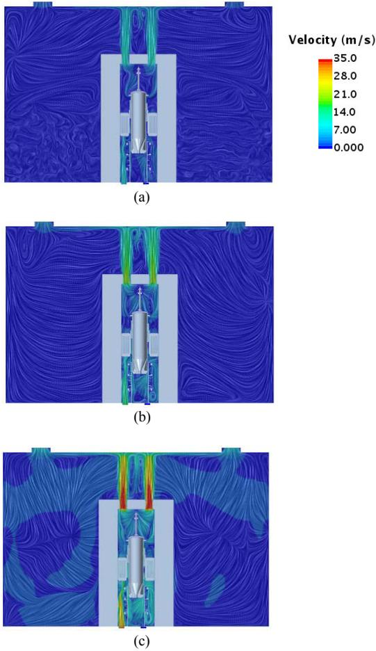
Fig. 2. Ex-core fluid velocity contours over XZ-plane. (a) 2 kg/s; (b) 4 kg/s; (c) 8 kg/s.
