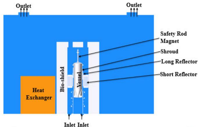
Fig. 1. Ex-core geometry configuration for forced-air cooling.
