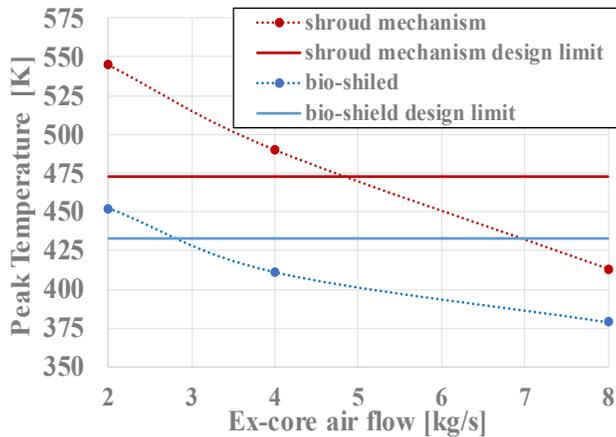
Fig. 5. Peak temperature in the bio-shield (blue dashed line) and shroud mechanisms (red dashed line) as a function of the air mass flow rate.
