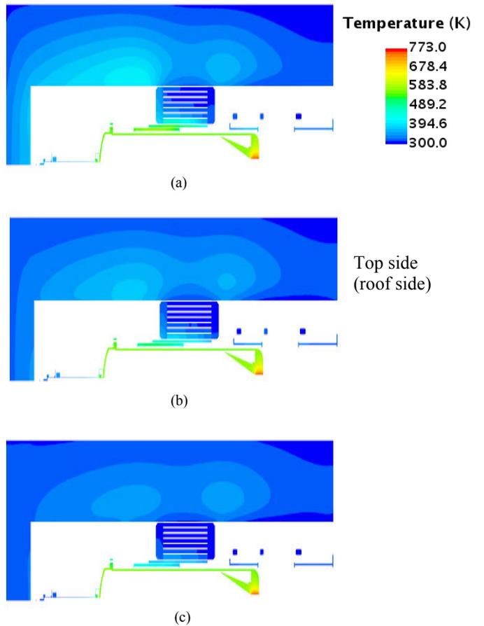
Fig. 4. Ex-core solid temperature distribution over vertical plane at center (YZ-plane) (rotated by 90°) for various inlet air coolant mass flow rates. (a) 2 kg/s; (b) 4 kg/s; (c) 8 kg/s.
