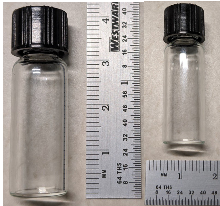
Figure 3. The 2 \text{ cm}^3 powder vial used for powder sampling within each build.
