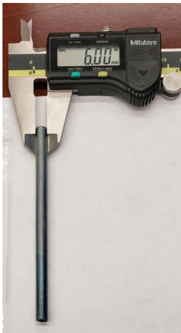
Fig. 4. As-fabricated YH x rod.
