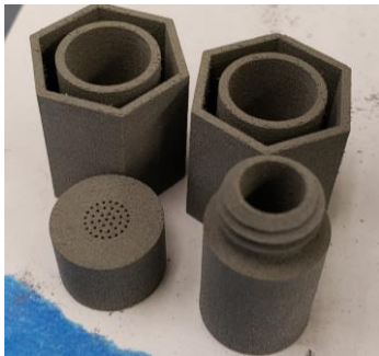
Figure 7: Green hexagonal compacts and Salt-Shaker Capsules for TREAT and MITR irradiations fabricated via Binderjet 3D printing
