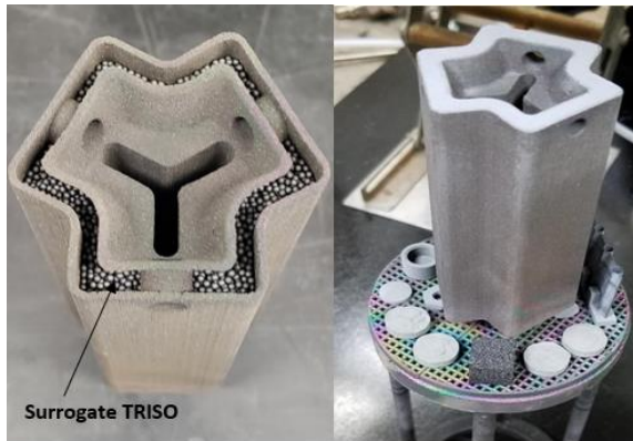
Figure 3: A Y-shaped fuel compact with built-in coolant pathways just before the final chemical vapor infiltration step
