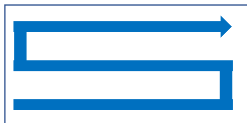
Figure 1: Snaking Laser Scan Strategy Used in Fabrication
