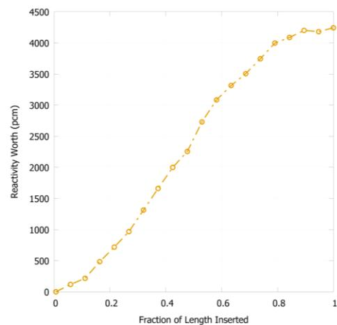
Fig. 4. Control shroud integral reactivity worth curve.
