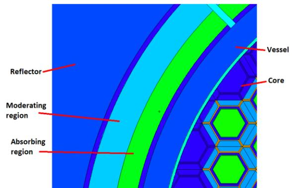
Fig. 3. Two-region control shroud configuration.
