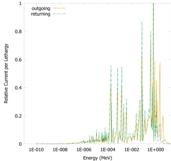
Fig. 2. Outgoing and incoming neutron current spectra in the control shroud region.
